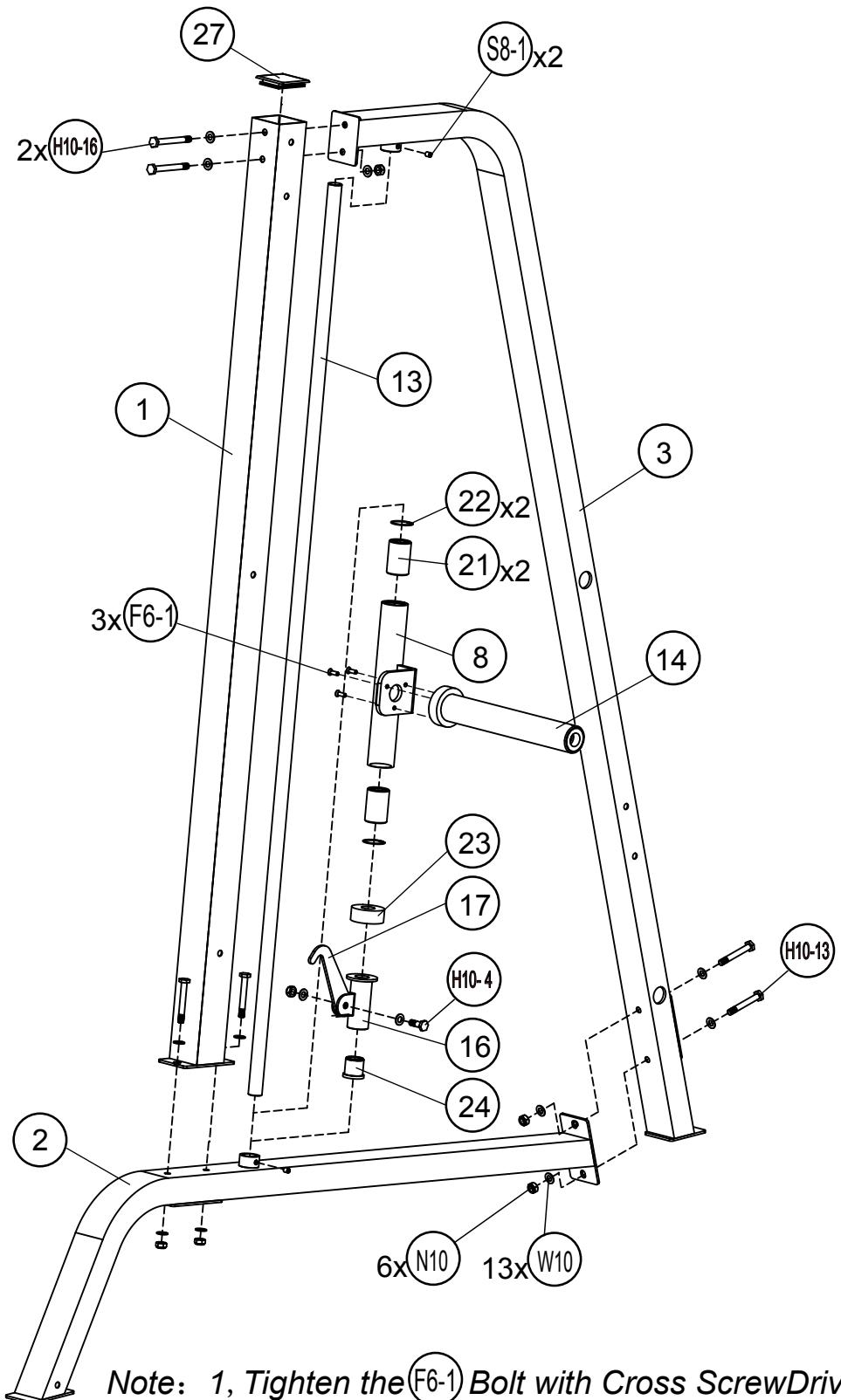
Note: 1, Tighten the F6-1 Bolt with Cross ScrewDriver;
